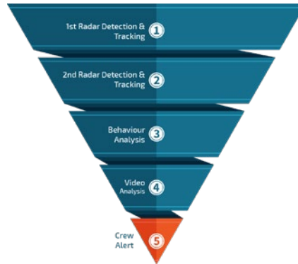
► FIG.4 The MARSS five-layer decision hierarchy leverages sensor redundancy for highest reliability.
